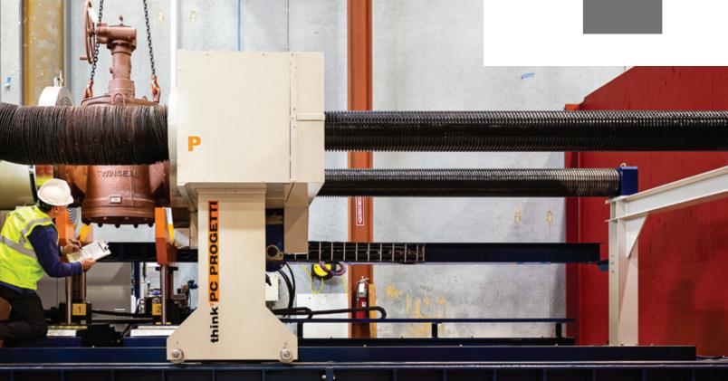
At our new Valve Engineering and Modification Center, a large double block and bleed expanding plug valve undergoes an extended duration hydrotest before delivery to a midstream pipeline installation.
