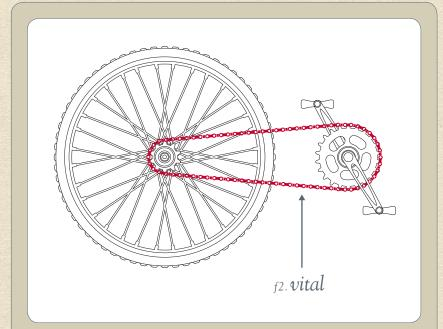
A bicycle chain is a vital component in the energy-efficient transfer of power from pedals to the drive-wheel, enabling continuous movement of the machine.
