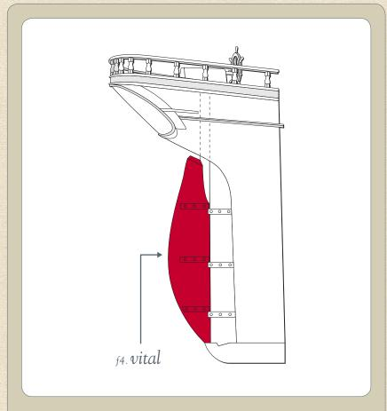
The rudder is one of the most vital components of a ship, without which, controlling the direction of the vessel would be impossible.
