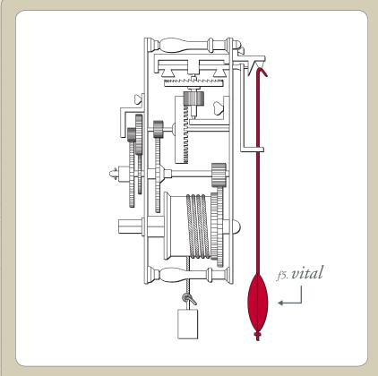
The pendulum is vital in maintaining constant movement in the mechanism of a clock, achieving an accurate measurement of time.
